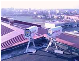
Two M1 ARTOLINK (MOSTCOM) wireless optical systems in Veseli na Morave (Czech Republic) - distances near 900 m
