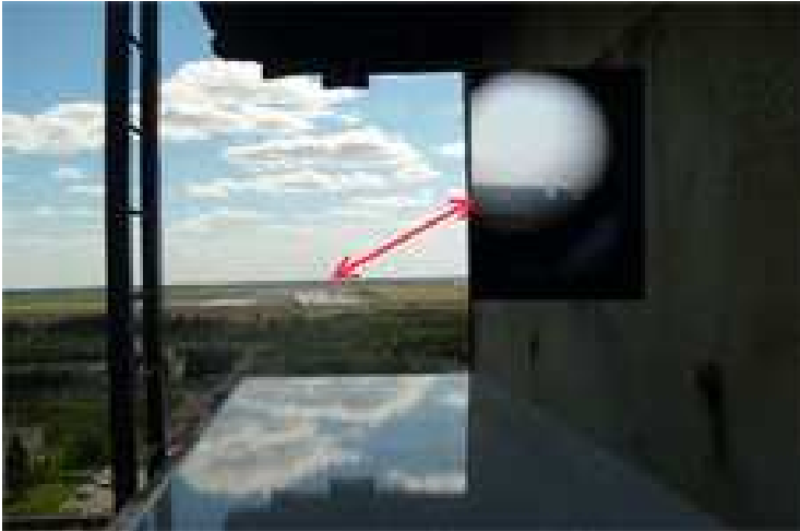
Wireless optical system M1 ARTOLINK (MOSTCOM) in Omsk - distance 6,7 km
