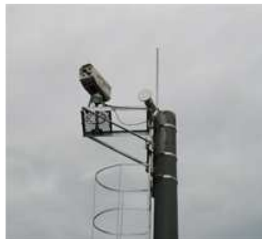
Hybrid wireless (FSO+MMW) link ARTOLINK M1 FE-R (MOSTCOM Ltd.) in Rostov region - distance 500 m
