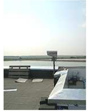
FSO equipment M1 ARTOLINK (MOSTCOM) in Naberezhnye Chelny - distance 1.2 km
