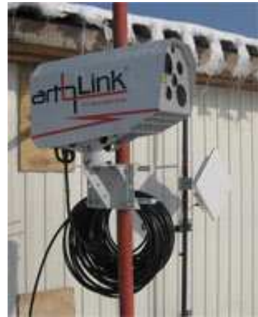
Free space optics system M1 ARTOLINK (MOSTCOM) in Moscow region - distance 1.6 km
