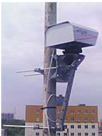
Wireless optical system M1 ARTOLINK (MOSTCOM) in Megafon company (Samara) - distance 120 m
