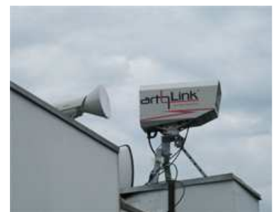
Hybrid wireless (FSO+MMW) link ARTOLINK M1 FE-R (MOSTCOM Ltd.) in Rostov region - distance 500 m
