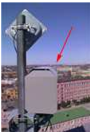
FSO equipment M1 ARTOLINK (MOSTCOM) in Ryazan - distance 5 km
